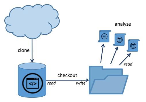
For every file: 2 read ops + 1 write op Checkout includes irrelevant files Need 1 CWD for every revision to be analyzed in parallel
