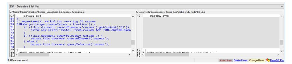
A function from the d3-node library which is not exercised by test cases and was removed by the optimizer.
